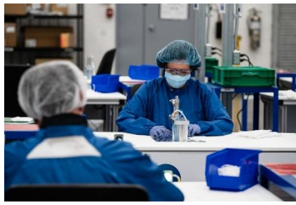
Workers assemble masks using ultrasonic welding stations which bind the ear strings to the mask material.
